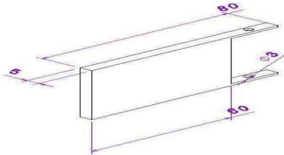
**Fig: 4.12 Valve head with dimensions Actual**
