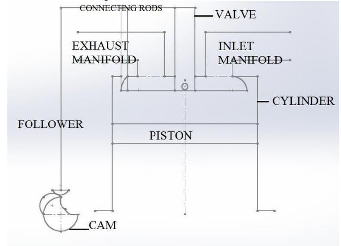
Fig: 4.1 Assembly of new engine
