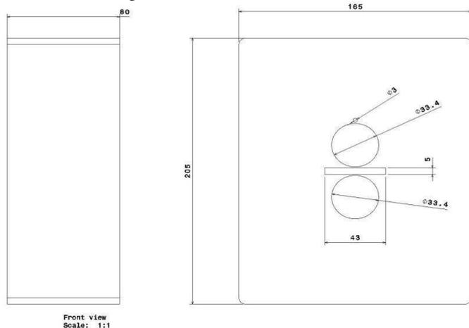
**Fig: 4.14 Cylinder head with dimensions**
